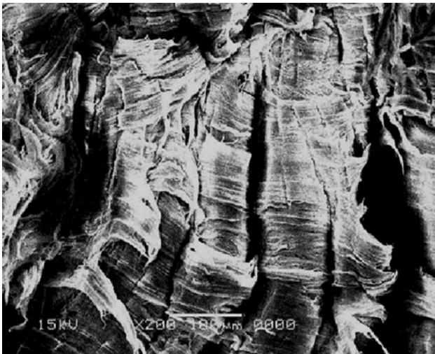
Fig. 7 SEM fractograph showing the HDPE sample fatigued at 40 °C and a frequency of 50 Hz
